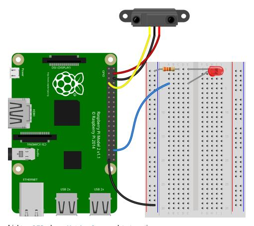
Light an  $\mbox{\it LED}$  when a  $\mbox{\it MotionSensor}$  detects motion:
