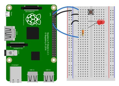
Turn on an LED when a Button is pressed:
