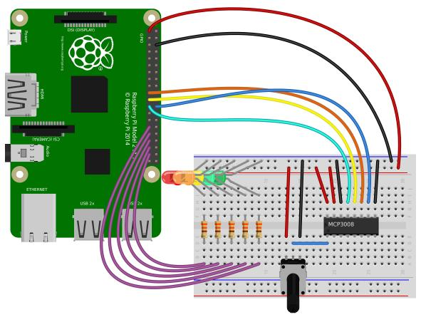
Continually print the value of a potentiometer (values between 0 and 1) connected to a MCP3008 analog to digital converter:
