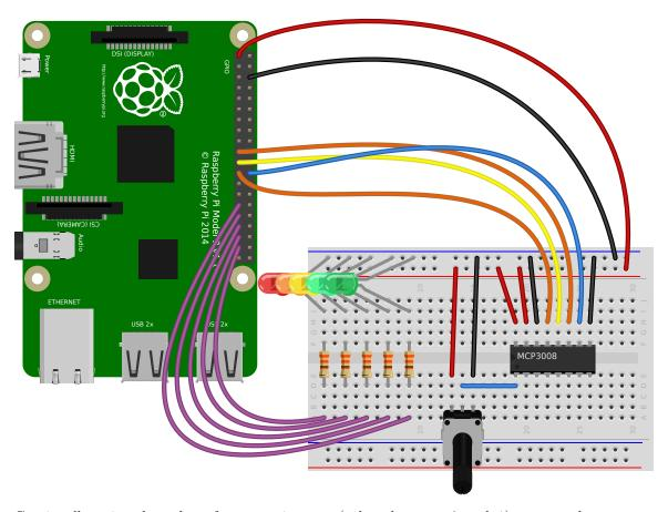
Continually print the value of a potentiometer (values between 0 and 1) connected to a MCP3008 (page 147) analog to digital converter:
