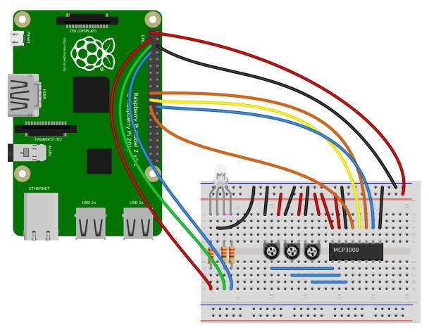
Wire up three potentiometers (for red, green and blue) and use each of their values to make up the colour of the LED:
