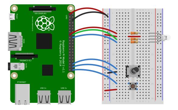
**Note:** In this recipe, I've used a common anode RGB LED. Often, Pi projects use common cathode RGB LEDs because they're slightly easier to think about electrically. However, in this case all three components can be found in an illuminated rotary encoder which incorporates a common anode RGB LED, and a momentary push button. This is also the reason for the button being wired active-low, contrary to most other examples in this documentation.
