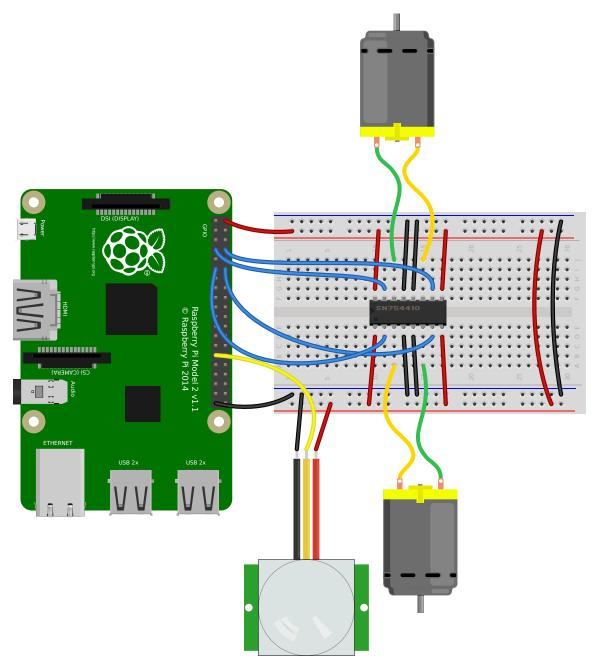
Make a robot drive forward when it detects motion:
