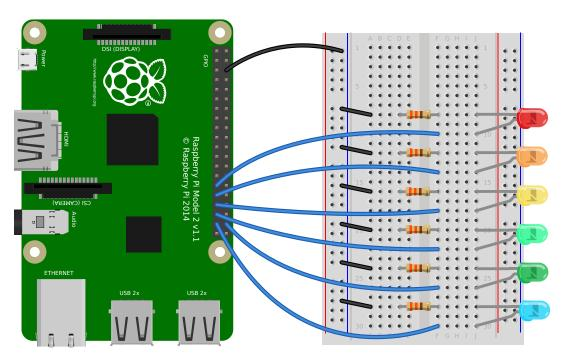
A collection of LEDs can be treated like a bar graph using LEDBarGraph (page 158):
