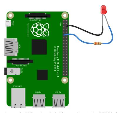
Any regular LED can have its brightness value set using PWM (pulse-width-modulation). In GPIO Zero, this can be achieved using PWMLED (page 125) using values between 0 and 1:
