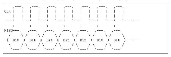
The following diagram indicates when data is read when  $clock\_polarity$  (page 236) is False  $^{1006}$ , but  $clock\_phase$  (page 235) is True  $^{1007}$ , equivalent to CPHA 1:
