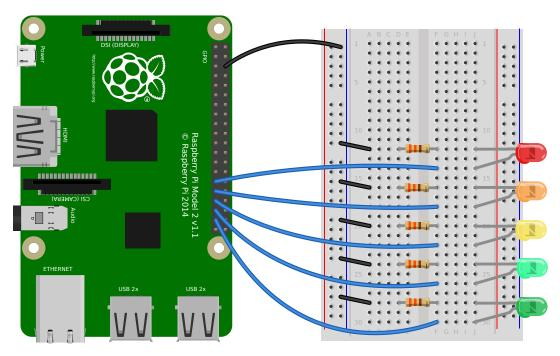
A collection of LEDs can be accessed using *LEDBoard* (page 155):
