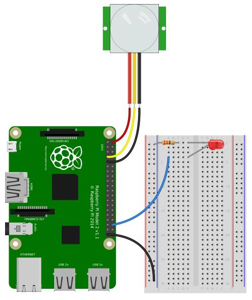
Light an  $\it LED$  (page 123) when a  $\it MotionSensor$  (page 108) detects motion:
