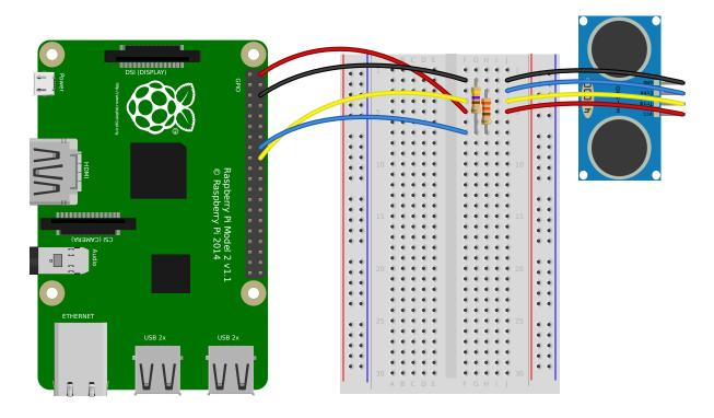
**Note:** In the diagram above, the wires leading from the sensor to the breadboard can be omitted; simply plug the sensor directly into the breadboard facing the edge (unfortunately this is difficult to illustrate in the diagram without the sensor's diagram obscuring most of the breadboard!)
