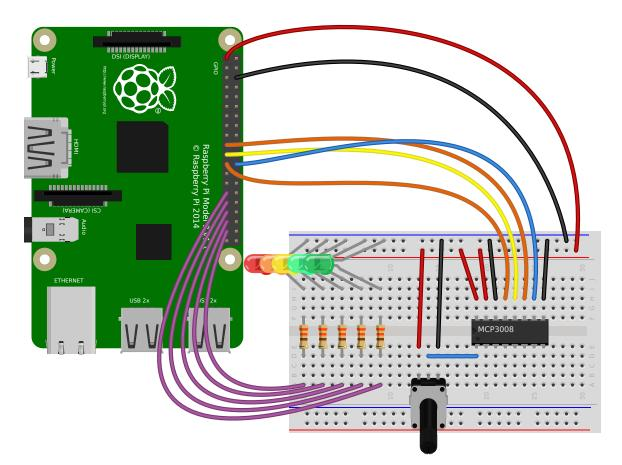
Continually print the value of a potentiometer (values between 0 and 1) connected to a MCP3008 (page 147) analog to digital converter:
