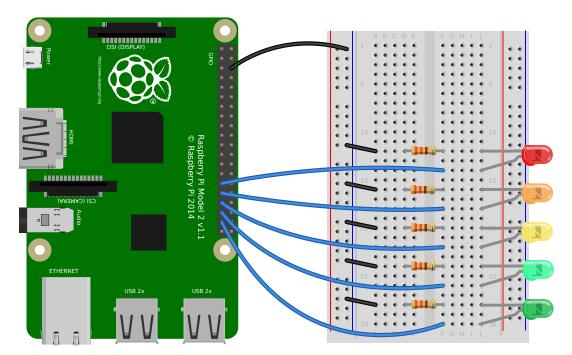
A collection of LEDs can be accessed using *LEDBoard* (page 155):
