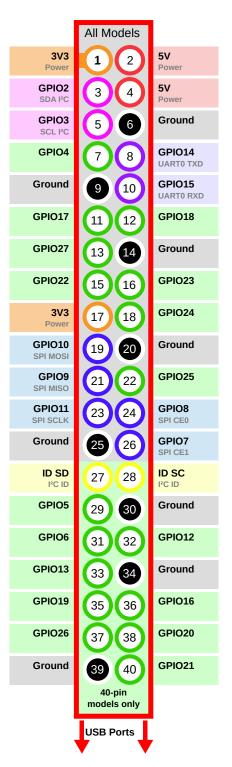
If you wish to use physical (BOARD) numbering you can specify the pin number as "BOARD11". If you are familiar with the wiringPi<sup>11</sup> pin numbers (another physical layout) you could use "WPI0" instead. Finally, you can specify pins as "header:number", e.g. "J8:11" meaning physical pin 11 on header J8 (the GPIO header on modern Pis). Hence, the following lines are all equivalent:
