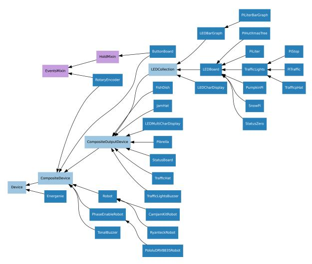
For composite devices, the following chart shows which devices are composed of which other devices:
