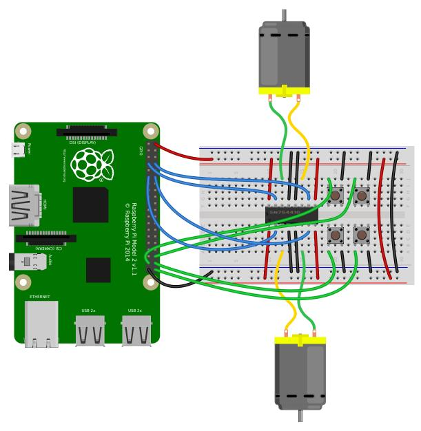
Use four GPIO buttons as forward/back/left/right controls for a robot:
