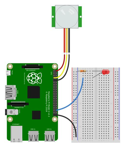
Light an *LED* (page 123) when a *MotionSensor* (page 108) detects motion:
