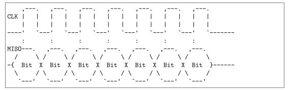
The following diagram indicates when data is read when *clock\_polarity* (page 236) is False<sup>1006</sup>, but *clock\_phase* (page 235) is True<sup>1007</sup>, equivalent to CPHA 1:
