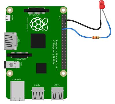
Any regular LED can have its brightness value set using PWM (pulse-width-modulation). In GPIO Zero, this can be achieved using *PWMLED* (page 125) using values between 0 and 1:
