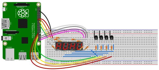
This circuit demonstrates a 4-character 7-segment (actually 8-segment, with decimal-point) display, controlled by the Pi's GPIOs with 4 2N-3904 NPN transistors to control the digits.
