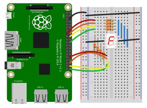
A common 7-segment display<sup>14</sup> can be used to represent a variety of characters using *LEDCharDisplay* (page 160) (which actually supports an arbitrary number of segments):
